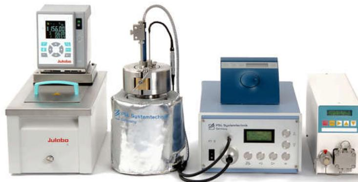
measuring station. The measuring station has an additional dosing pump for titrating the sample as well as a thermostat. The latter enables measurements at high temperatures to distinguish paraffin and asphaltene precipitation.
