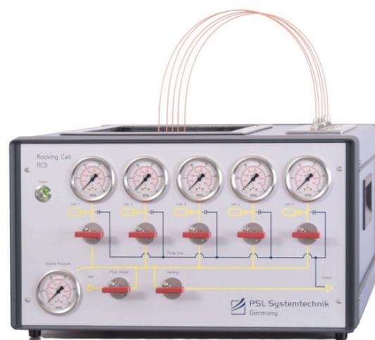
2. Shut-in: The test chambers are kept in a given position (adjustable up to 45° angle). The sample is cooled or heated to scheduled temperature.
