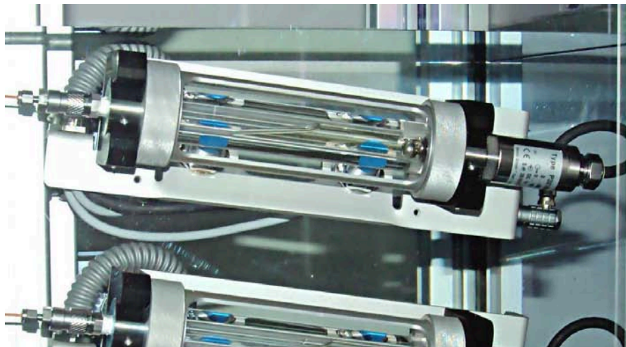
Detail: Mounted sapphire test cell in cooling liquid
